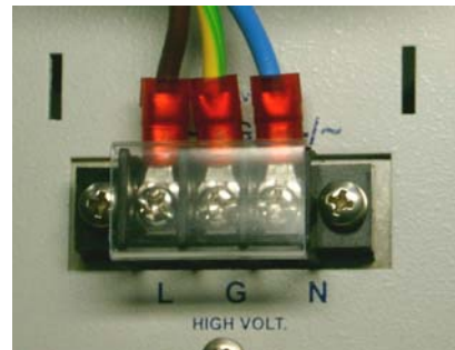
Fig. 6.4: Power Terminal Block Locked
